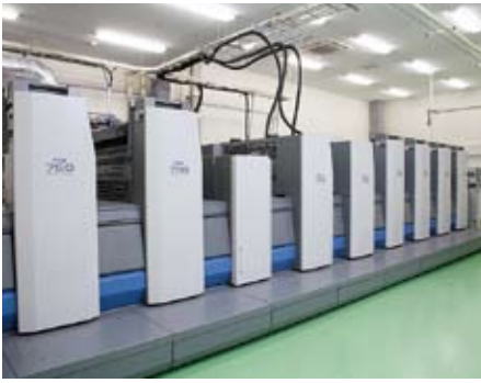
World's first inline UV press with 3 Kodak Prosper S5 Imprinting Systems
